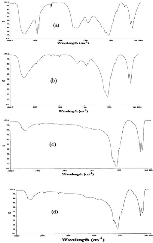
**Fig. 1** FT-IR spectra of fishbone heated at (a) 100°C (b) 400°C (c) 700°C (d) 900°C
