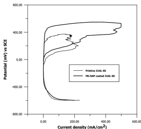
**Fig. 3 Cyclic polarisation curves of pristine and fishbone-originated HAP coated 316L SS in Ringer's solution**
